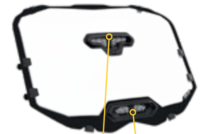
Upper vent channels air into the cabin
